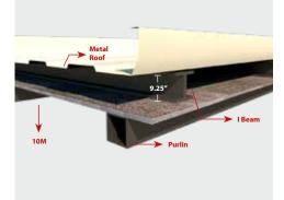
➔ Tested in bays ranging between 8 to 13 ft. No issue spanning large bays.
